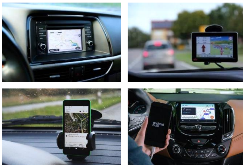
Figure 11 Types of navigation systems (from top left to bottom right): a built-in navigation system, a nomadic navigation system, a smartphone with a navigation application, and an app displayed on the dashboard (Apple CarPlay, Android Auto).
